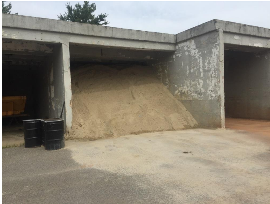
Figure 3: Improper Sand Storage – Sand should be swept up and exposed pile covered, stored further under cover or inventory reduced
