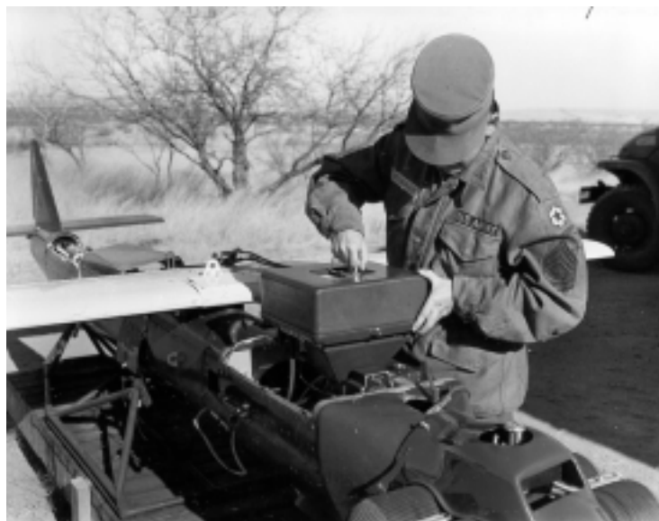
1956.00.00.013 SFC Kenneth R. Bridgham, Photographic and Television Division, Battle Area Surveillance Department, Fort Huachuca, installing a KA20 aerial reconnaissance camera in an RP-71 drone aircraft. U.S. Army photo.
