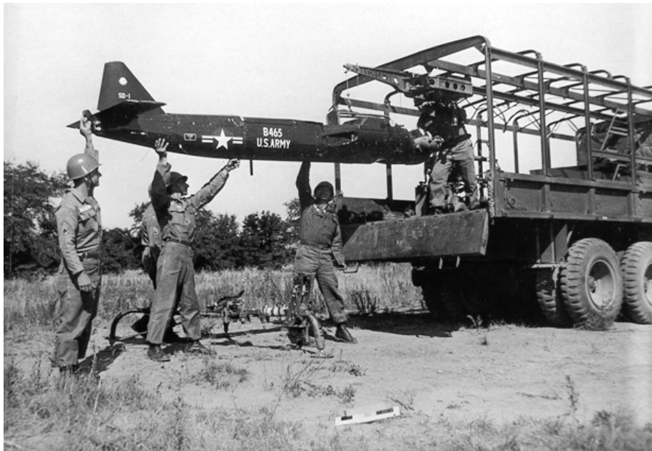
Loading a SD-1 drone on a 2 1/2-ton truck in the 1960s. U.S. Army photo.
