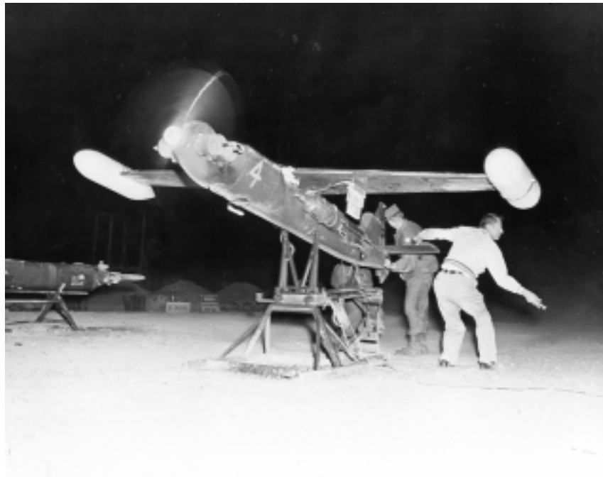
Checking controls of the RP-71 drone just before takeoff at Fort Huachuca in the 1960s. U.S. Army photo.
