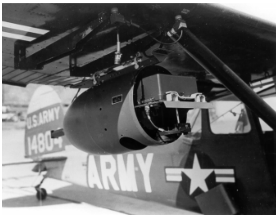
Surveillance camera pod mounted on Army reconnaissance aircraft.
