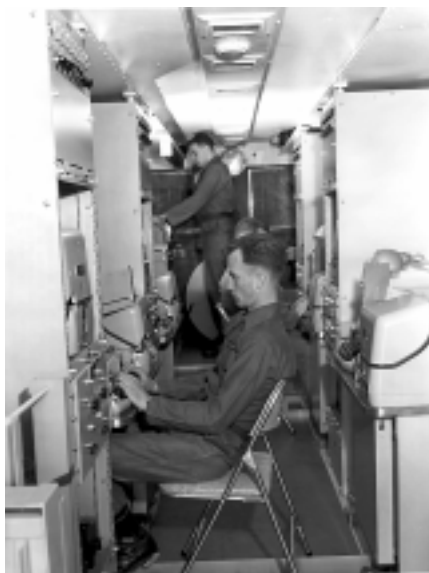
Army air-ground transportable, radio communications system, the AN/TSC-16, is geared to quick-reaction demands of small wars and brush-fire combat operations by elements of STRAC. The system consists of transmitter van, comcenter-receiver van, and power unit. The equipment was built by Adler Electronics, Inc, New Rochelle, NY, based on specifications prepared by the U.S. Army Signal Engineering Agency. Working in the comcenter-receiver van are Pfc. Northam B. Jefferies, seated at the teletypewriter in the foreground, and Pvt. Ronald W. Rotondo, standing in the rear of the van. U.S. Army Signal Corps photo SC547484.
