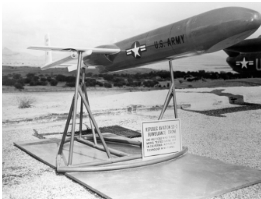
A 1/2-scale wind tunnel model of the Republic Aviation SD-3 Surveillance Drone.
