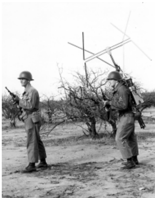
Soldiers wearing the experimental model of the Manpack Jammer EP/EDL-39 in 1960. U.S. Army photo.
