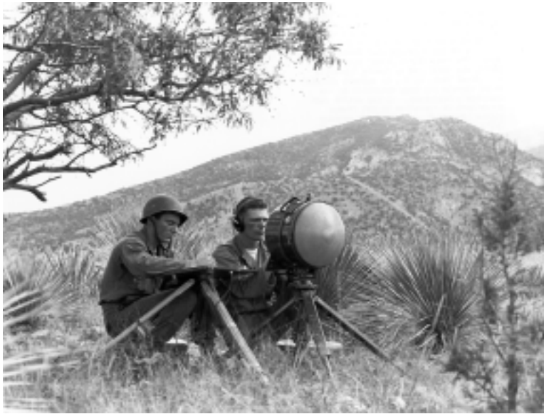
Daylight view of the Army's new compact, all-weather radar "eye" (AN/PPS-4 Radar Set) which can spot a single enemy moving a half-mile away in darkness or fog, vehicles or large groups much farther away. It is operated by Pvt. Thomas Hughes, while Pvt. Anthony Devlin tracks the "enemy" movement on plotting board as latest protection in forward combat zones. U.S. Army photo.
