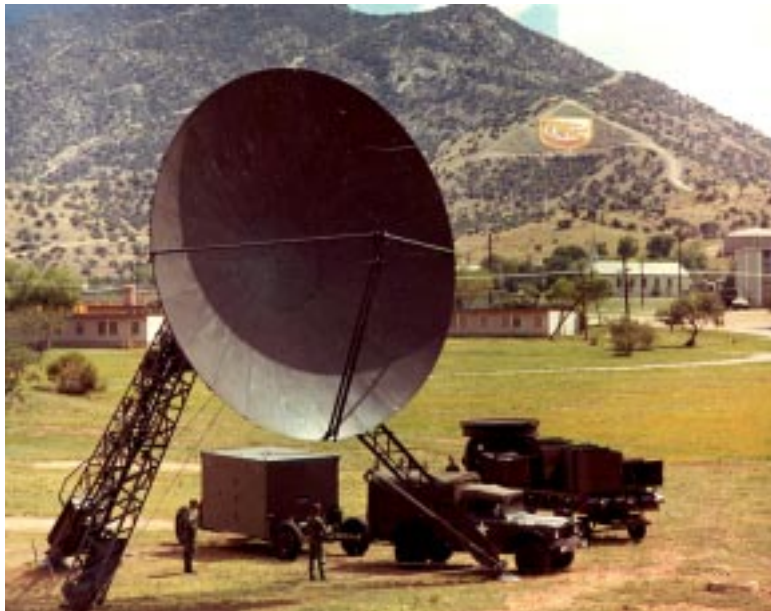
Troops of the 11th Signal Group, U.S. Army Strategic Communications Command (STRATCOM), set up the Radio Terminal Set (Heavy Tropo) at Fort Huachuca in July 1968. U.S. Army photo.
