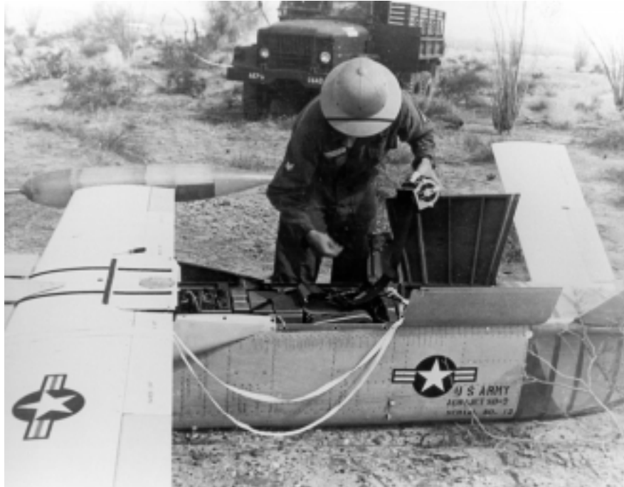
The film being removed from an Aerojet Surveillance Drone-2 at Huachuca's ranges. U.S. Army photo.
