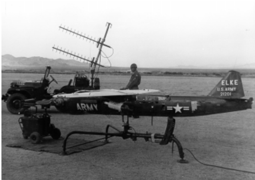
A surveillance drone being tested on Huachuca's ranges by USAEPG. U.S. Army photo.
