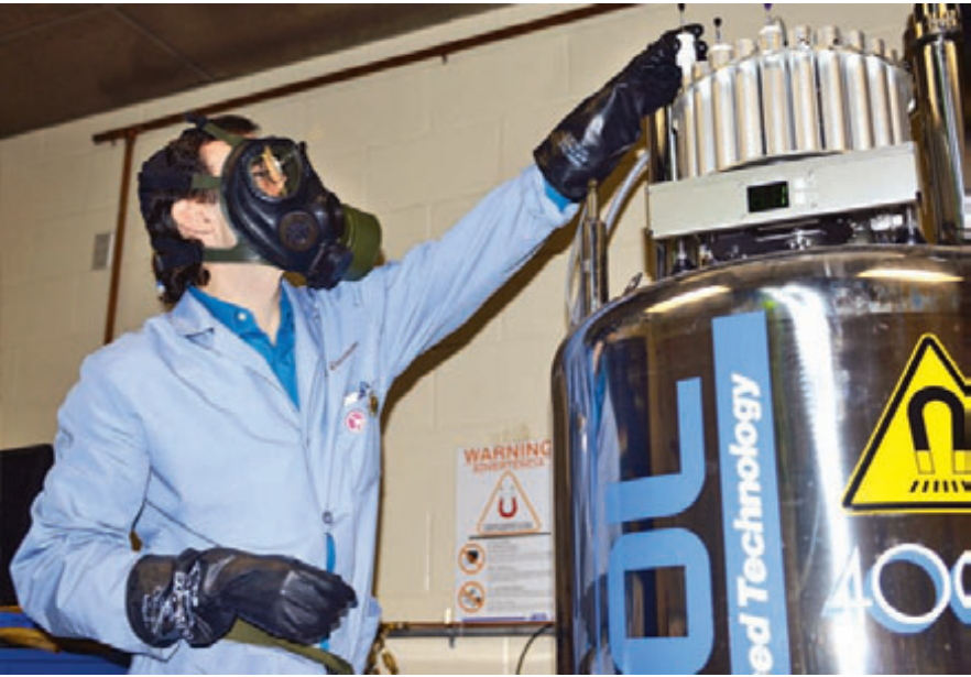
Chemist David McGarvey, Ph.D., of the Army’s Edgewood Chemical Biological Center, on Aberdeen Proving Ground, inserts a swatch of fabric into a nuclear magnetic resonance spectrometer.
