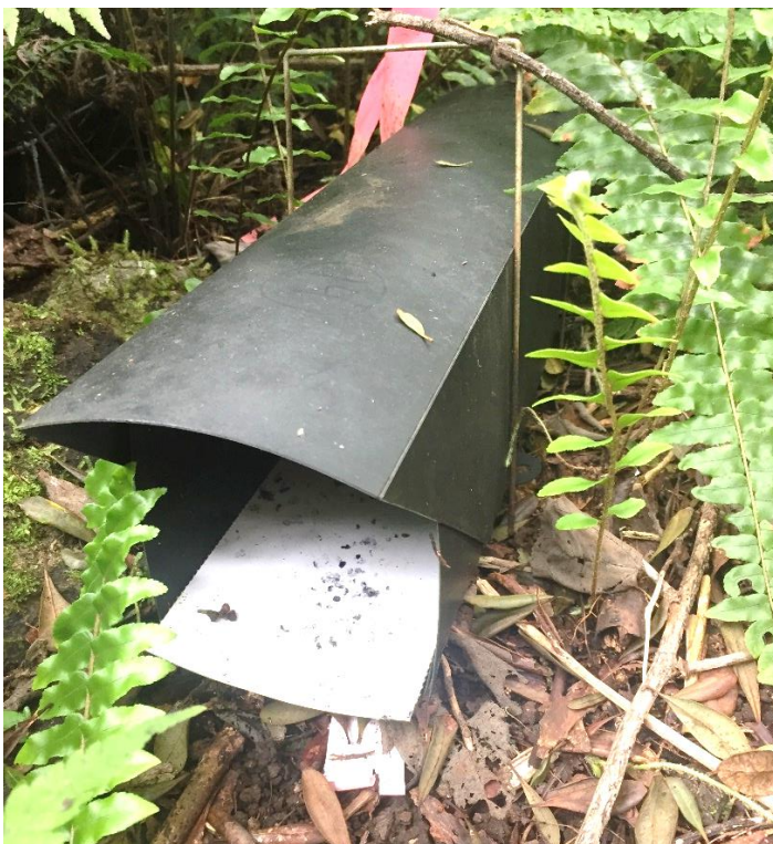
Tracking Tunnel and Ink Card with Rat Tracks
