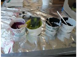
Step 3: The mixing table must be checked, at a minimum, at the end of each work shift. Any mixing cups and applicators that are no longer usable must be collected and turned in to the ECO immediately. DO NOT PLACE AVIATION MAINTENANCE DEBRIS IN THE USED AVIATION RAGS CONTAINERS!
