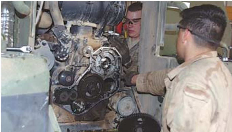
Pfc. Jason Sumner (near, right) and Spc. Rockwell Phillips, both Soldiers with Headquarters Support Company, 209th Aviation Support Battalion, Task Force Lobos, 25th Combat Aviation Brigade, replace engine seals on an up-armored vehicle at Contingency Operating Base Speicher, near Tikrit, Iraq, March 9.
