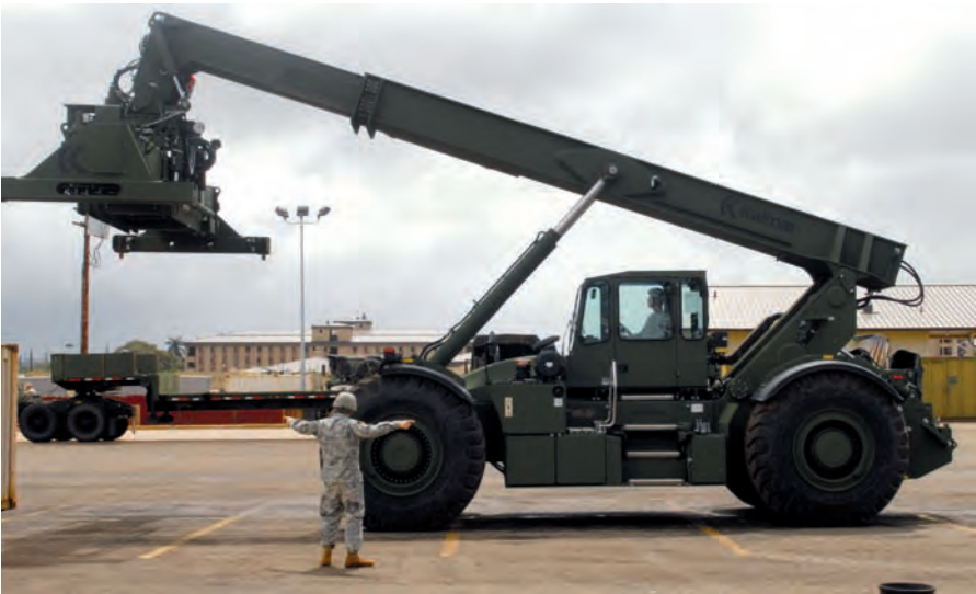
Pfc. Kyle Calkins, automated logistical specialist, operates the RTCH, while Pvt. Sean Fett, automated logistical specialist, both in 40th Quartermaster Co., 524th CSSB, 45th Sust. Bde., 8th TSC, ground-guides him through the specific movements of the vehicle.
