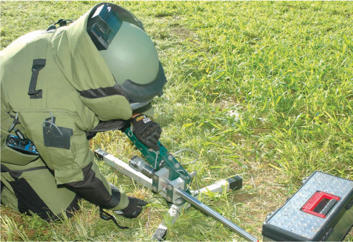
Staff Sgt. Justin Talbert, team leader, 706th EOD Co., 303rd EOD Bn., 45th Sust. Bde., 8th TSC, aims the Percussion Actuated Neutralizer at the suspected IED to defeat the device from its intended purpose of detonation.
