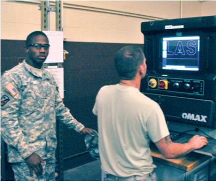
Air Force Staff Sgt. James Mattingly (right), from the 15th Maintenance Sqdn., shows Spc. Raymond Ramos-Fee, FSC, 65th Eng. Bn., 130th Eng. Bde., 8th TSC, how to format shape cutouts with the CNC Jet-Cutting machine.
