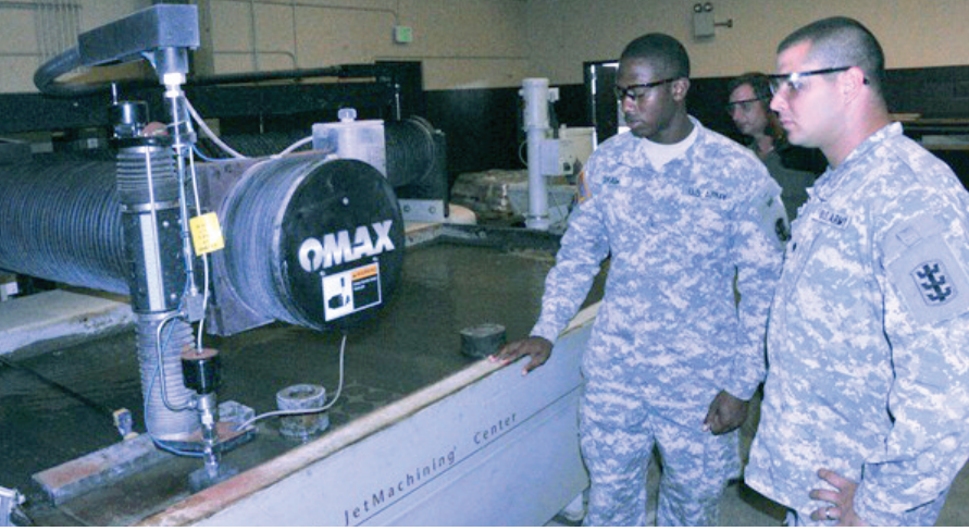
Sgt. Anthony Shaw (left) and Spc. Raymond Ramos-Fee, both with FSC, 65th Eng. Bn., 130th Eng. Bde., 8th TSC, watch as the CNC Jet-Cutting machine slices a piece of aluminum. The water jet machine is accurate to within three human hairs.
