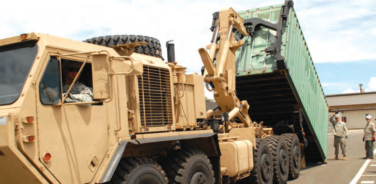
Spc. Russell Gray (driving), motor vehicle operator, 25th Trans. Co., 524th CSSB, 45th Sust. Bde., 8th TSC, operates the PLS-A1 and E-CHU, as Spc. Brian Percy, 25th Trans. Co., 524th CSSB, 45th Sust. Bde., gives proper hand signals for the loading and unloading of a container.
