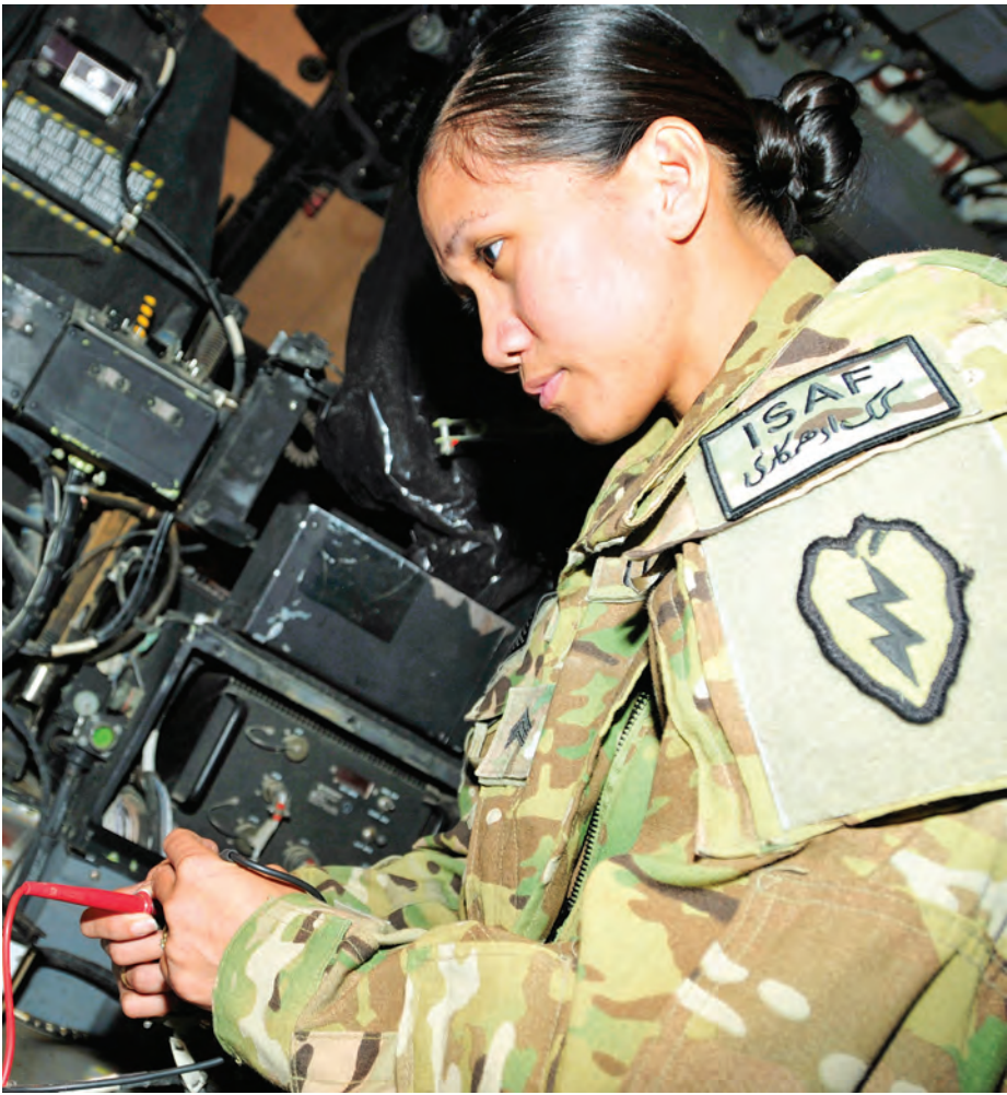
Sgt. Daniel Schroeder | 25th Combat Aviation Brigade Public Affairs Sgt. Grena Kirk, aircraft electrician, Co. B, 209th ASB, 25th CAB, checks a cannon plug as part of a phase maintenance inspection, Nov. 8. Kirk was sworn in as a U.S. citizen, at Bagram Airfield, Afghanistan, Nov. 2.
