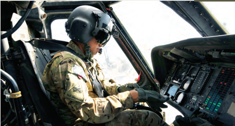
Chief Warrant Officer 3 Jerald Jastillama, maintenance test pilot, Co. A, 3rd Bn., 25th Avn. Regt., 25th CAB, 25th ID, performs a maintenance operational run-up of a UH-60 Black Hawk helicopter, Feb. 28.
