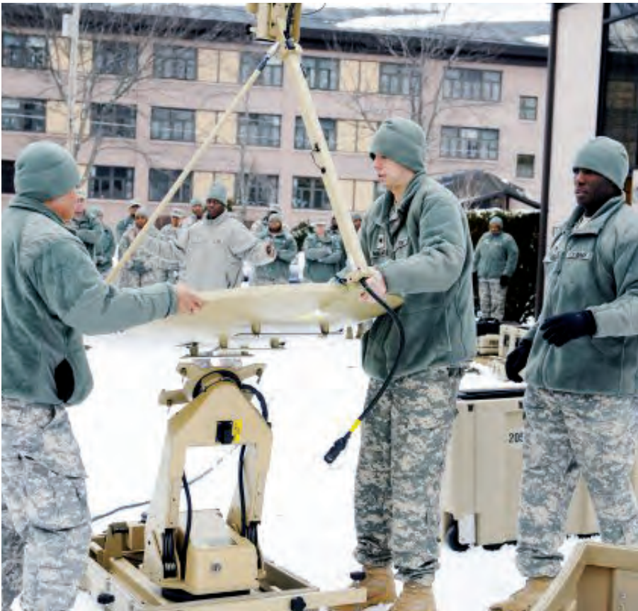
Staff Sgt. Atavis Taylor (right), second shift officer in charge, Casualty Operations, 14th HRSC, assists two Soldiers from the 8th HRSC, 8th TSC, in assembling the VSAT system during Silver Scimitar 2012. VSATs provide critical connectivity in an austere environment when other options are not available.
