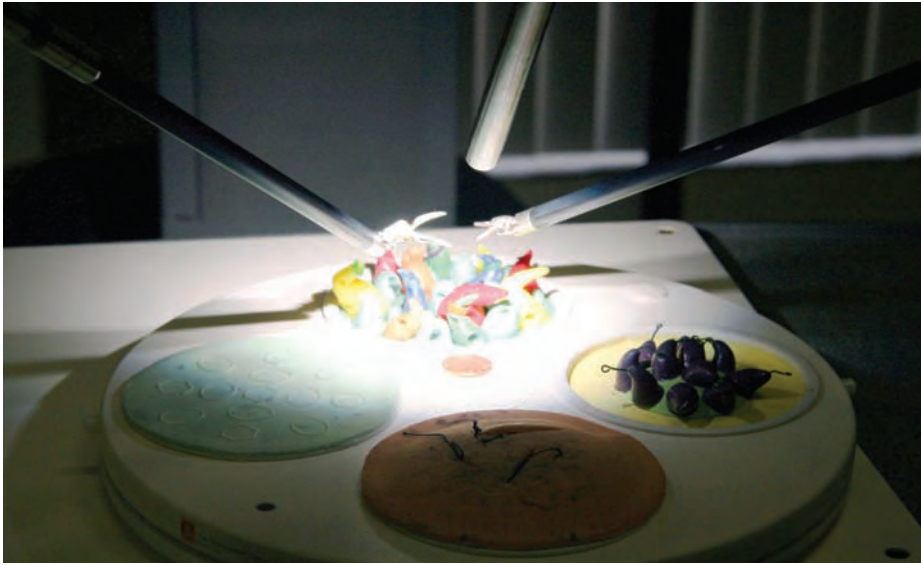
A simulation tool is set off on the da Vinci Surgical System table for surgeons and residents to practice on. The surgeon sits at the console and looks through two eye holes at a 3-D image of the procedure, while maneuvering the arms with two foot pedals and two hand controllers.
