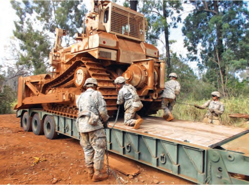
Soldiers of 4th Platoon, 95th Engineer Company (Clearance), 84th Eng. Battalion, 130th Eng. Brigade, 8th Theater Sustainment Command, attach the first set of chains used to secure a T9 dozer to a trailer during transport from the South Range engineering training area, here, earlier this month.
