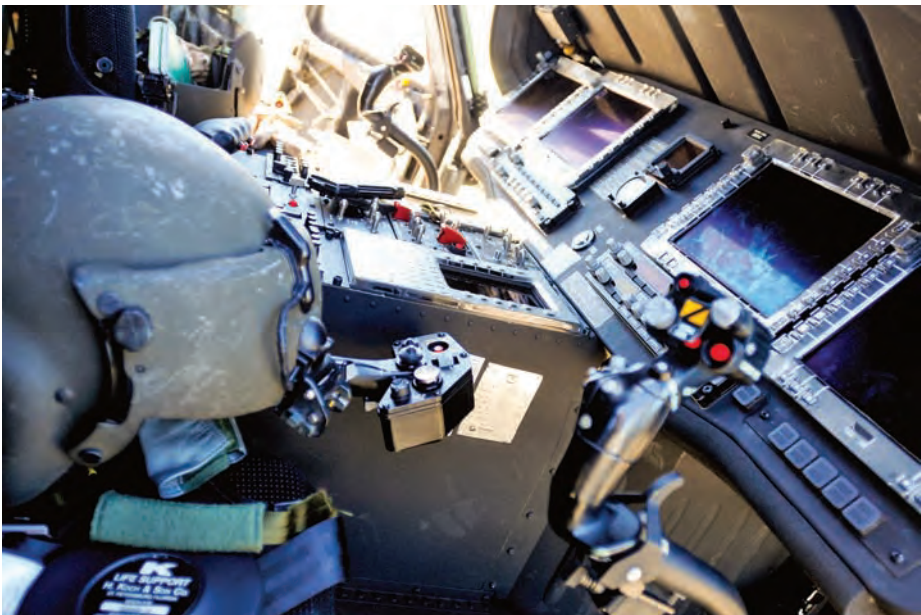
(Top and above) The UH-60M Black Hawk incorporates a glass cockpit that provides 25th CAB aircrews with increased situational awareness to better support Soldiers on the ground.
