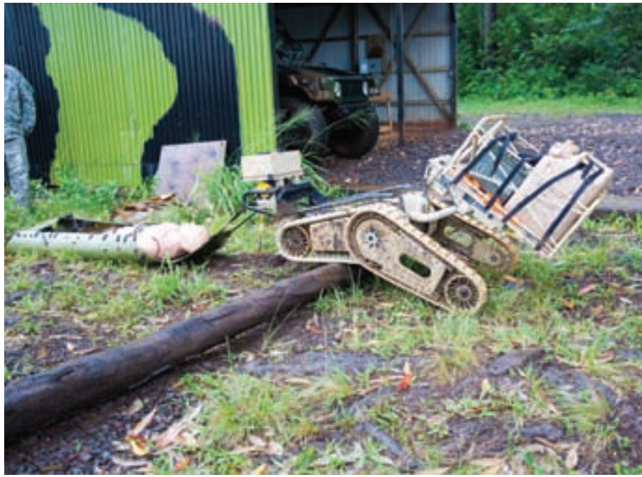
A robot being tested by Tropic Lightning Soldiers and RDECOM representatives at East Range tows a simulated casualty on a Skedco across uneven terrain, freeing up troops to stay in a fire-fight instead of carrying a wounded comrade to safety.
