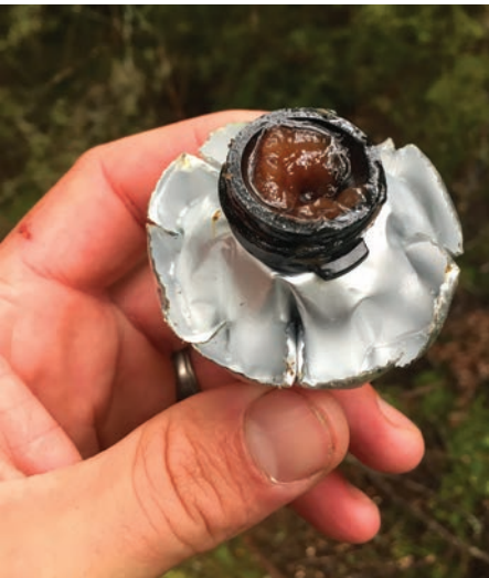
The self-resetting traps use an automatic lure pump, shown here, to release small amounts of chocolaty bait to attract invasive rats.
