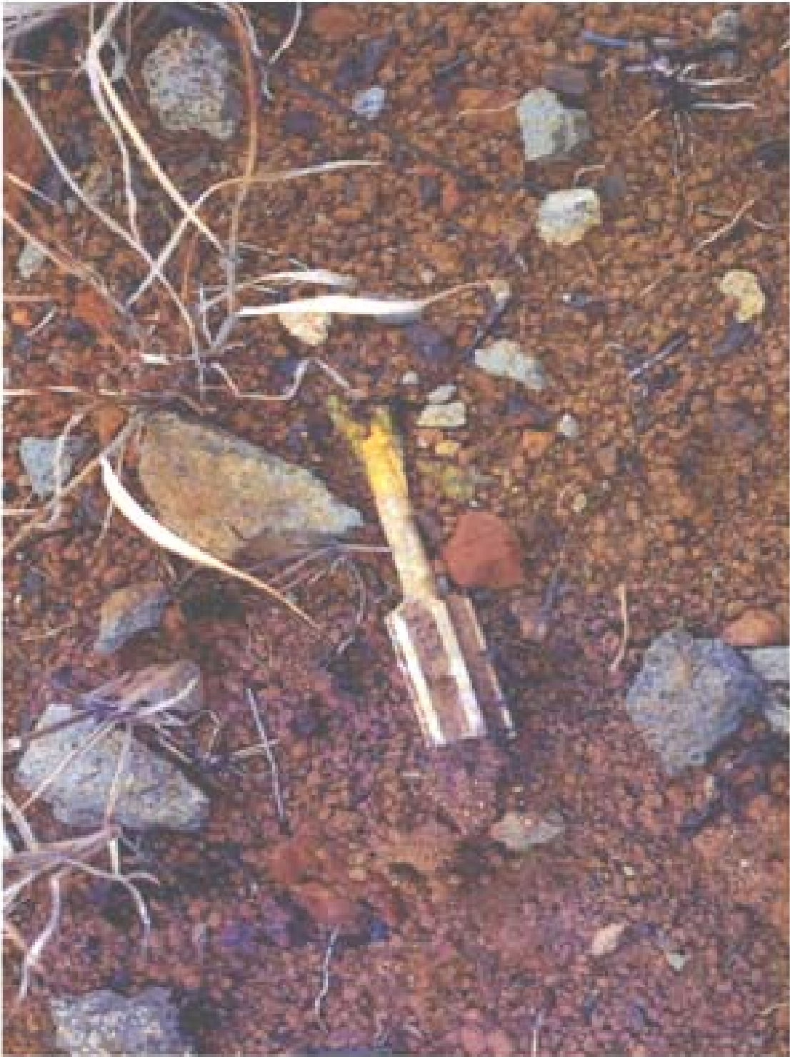
(11) Tail with Fins of Cartridge, 20mm Spotting M101 – Schofield Barracks
