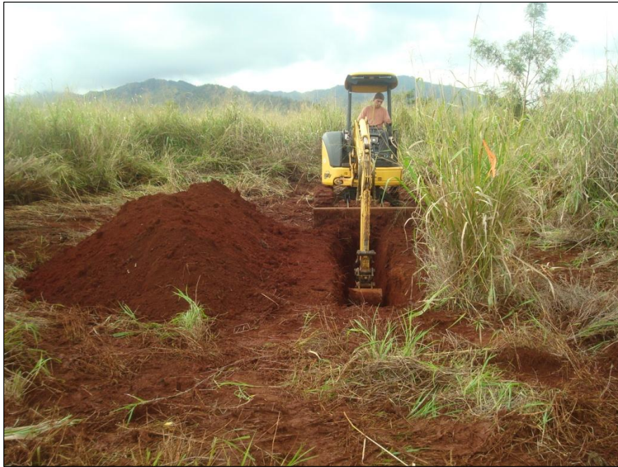
Figure 13. Komatsu PC35MR backhoe excavating at Trench 3.
