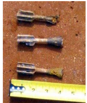
Tail assemblies belonging to the M101 spotting round. The yellow uranium oxide can be seen on the right side of the assembly. Note the small size of these items.
