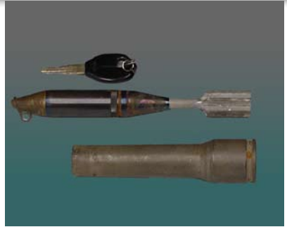
M101 spotting round and cartridge case—key shown for scale
