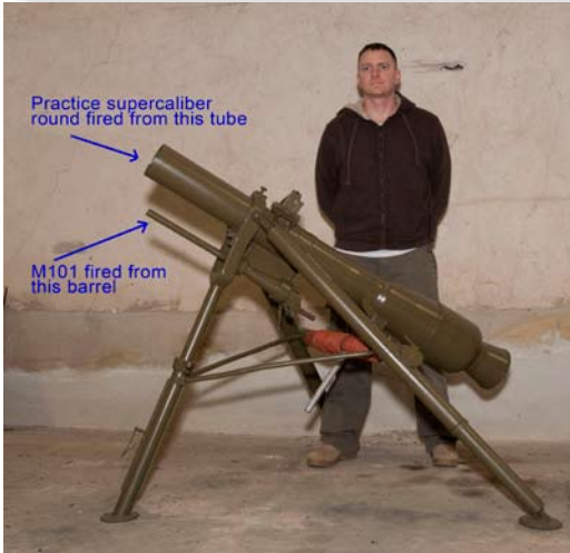
Davy Crockett M28 light weapon - note size of barrel that fired the M101
