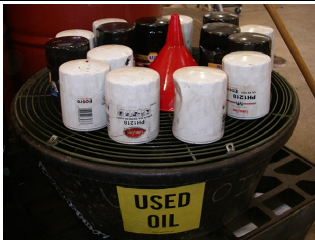
Proper Used Oil Filter draining station marked “USED OIL” and protected with secondary containment.
