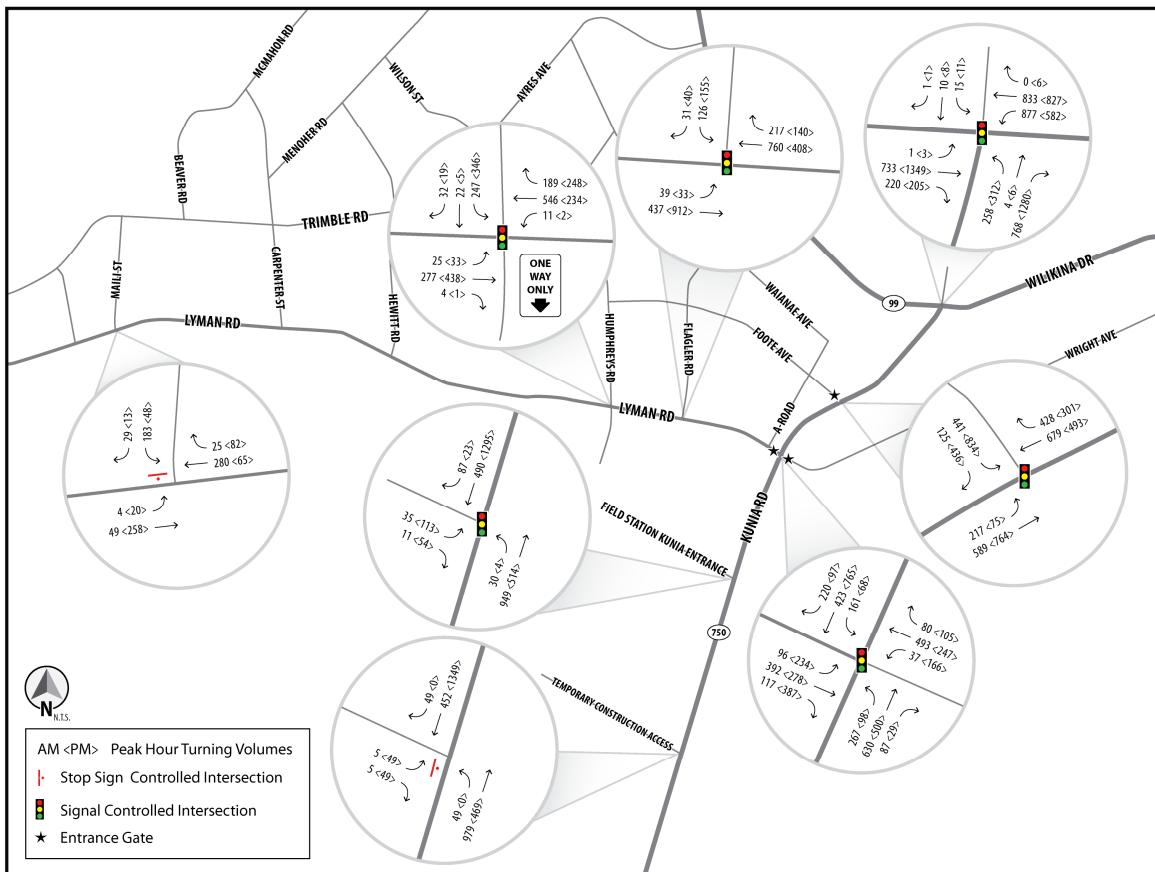
**Figure 6. 2017 Peak Hour Traffic Volumes During Construction**
