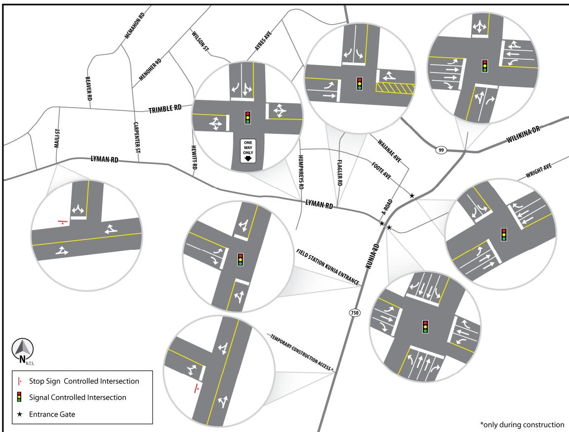
**Figure 4. 2017 Intersection Channelization**
