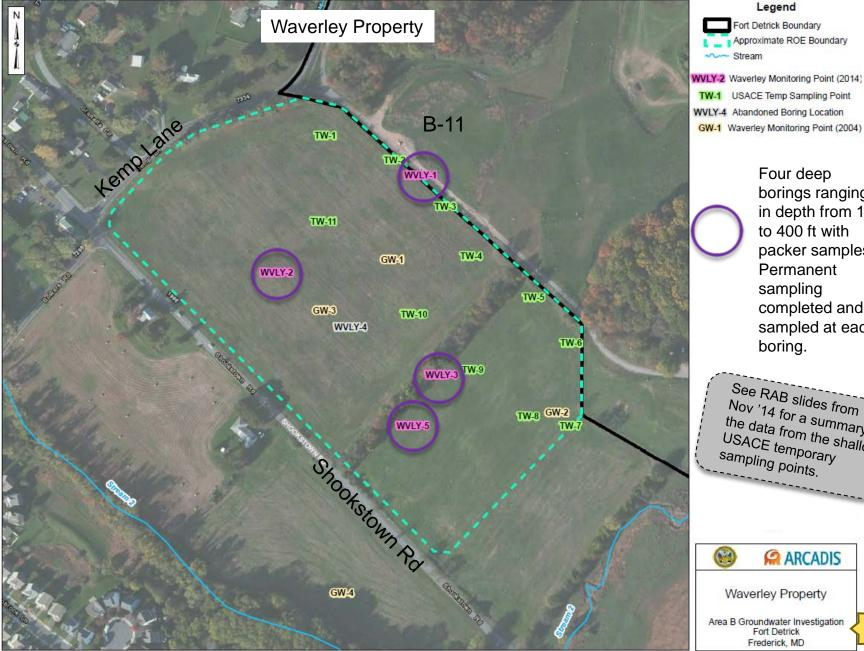
GW-1 Waverley Monitoring Point (2004) Four deep borings ranging in depth from 140 to 400 ft with packer samples. Permanent sampling completed and sampled at each boring.
