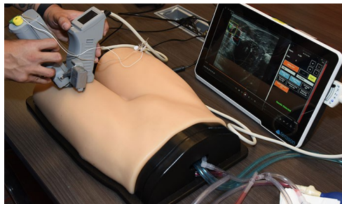
The prototype of an AI-enhanced ultrasound nerve block device developed by the U.S. Army Institute of Surgical Research Organ Support and Automation Technologies team in partnership with MIT is demonstrated on a manikin. (Photo by USAISR Public Affairs Office)
