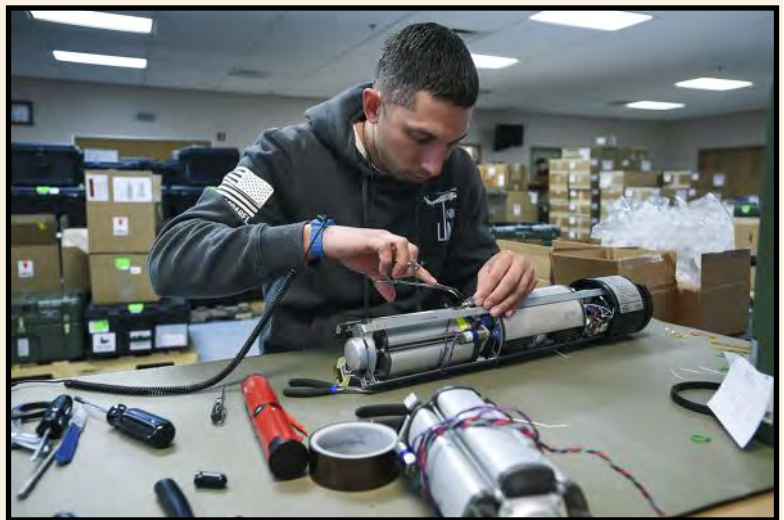
Matt Hernandez repairs an Oxygen Generator Field Portable, or OGFP (Model: 3000, NSN: 3655-01-648-5957, LIN: P05027), at the U.S. Army Medical Materiel Center Medical Maintenance Operations Division at Hill Air Force Base, Utah, Jan. 10, 2018.
