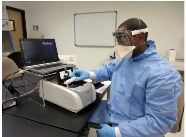
A Soldier demonstrates the use of the Warrior Panel, a DOD-funded diagnostic test, on the Next Generation Diagnostics System 1 (NGDS 1), known commercially as the BioFire® FilmArray®, which is used in hospitals and clinical settings around the world for standard health care diagnoses. Photo courtesy of JPM CBRN Medical.
