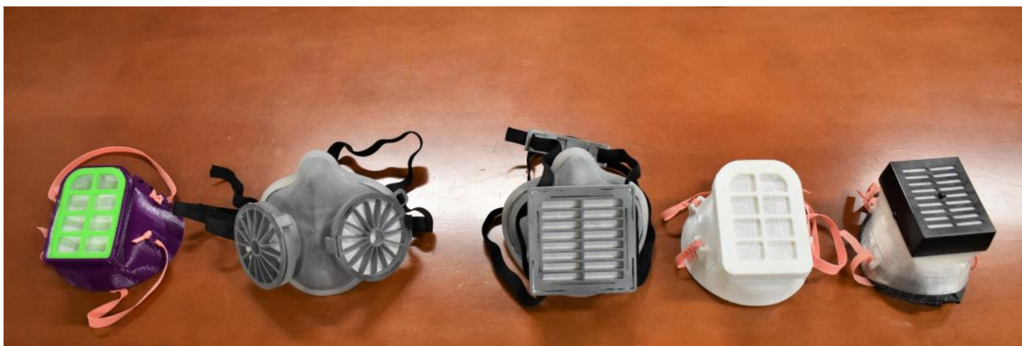
The U.S. Army Medical Materiel Development Activity's Warfighter Expeditionary Medicine and Treatment Project Management Office is involved in the DOD's effort to produce N95 respirators. Shown here are various prototypes of N95 masks that have been considered for production. These particular examples are elastomeric half-mask respirators, which have a reusable frame produced by a 3D printer, with a disposable media or cartridge that filters at the 95-percent level. The three masks on the right are early prototypes, while the two on the left are currently in the test and evaluation phase of development. (Photo by Jeffrey Soares, USAMMDA public affairs)
