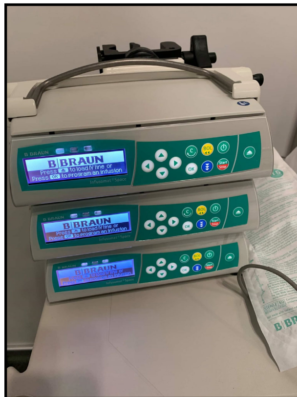
Army configuration for the Intravenous Infusion Pump Kit, which consists of three daisy-chained B. Braun Infusomat Space 2nd Generation infusion pumps.
