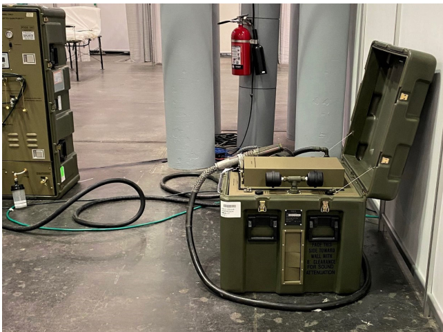
The POGS 33 unit uses the latest Pressure Swing Adsorption technology, and utilizes Zeolite Molecular Sieves to separate oxygen from the other gases contained in air. Used at the Javits Center in New York City during the U.S. Army's COVID-19 response.
