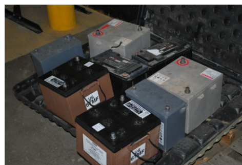
Batteries stored off the ground.
