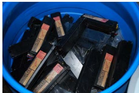
Ballasts and capacitors may contain PCBs and must be disposed of properly.
