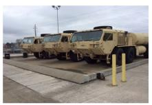
Drive-on containment (DOC) units are for containing accidental spills and preventing releases to the environment, not fueling or storing leaking equipment. Spills released into the DOC must be removed immediately for regulatory purposes. Additional spill assistance/guidance may be obtained from the Environmental Division Spill/Storage Tank Program, 270-798-9637/9601.
