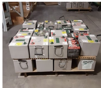
Batteries emit Hydrogen gas and could leak acid.
