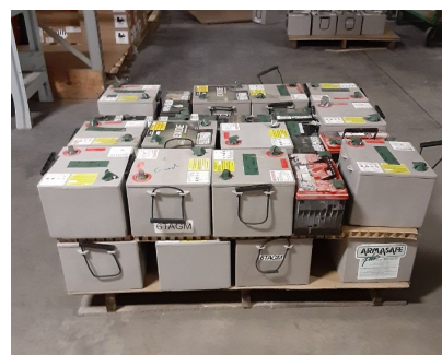
Batteries emit hydrogen gas and could leak acid. Secondary containment and proper ventilation is required.
