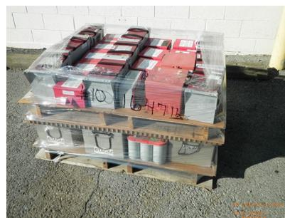
**Batteries emit hydrogen gas and could leak acid. Secondary containment and proper ventilation is required.**
