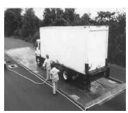
Vacuums/Pumps – Devices such as wet/dry vacuums, sump pumps, and vacuum pumps may be used to collect wastewater after pressure washing. Vacuum devices typically have an extension (vacuum boom) which allows the wastewater to be collected efficiently. In addition, many vacuum devices are designed with a second hose (e.g. garden hose) that can run from the pump to the sanitary sewer or a truck/trailer mounted holding tank, depending on disposal method.
