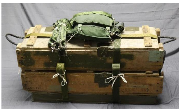
Figure 12.24c – Properly Rigged 68-Inch Pilot Parachutes with the A7-A Cargo Sling
