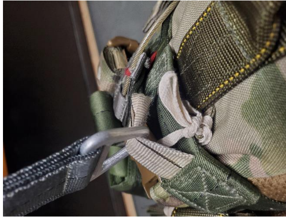
Figure 12.6an – Utilize 1/4" Cotton Webbing as the Point of Attachment
