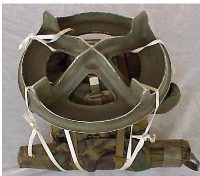
Figure 12.16s – Secure M7 Large Baseplate to ALICE Pack with Tubular Nylon
