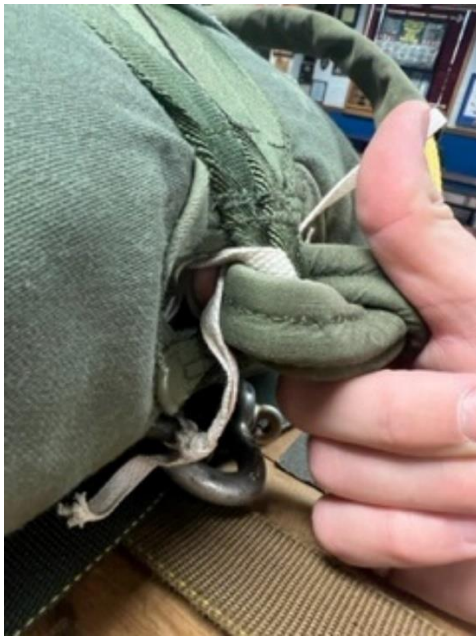
Figure 12.23b – Routing 1/4" cotton webbing
