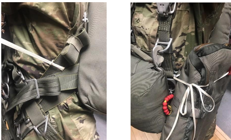
Figure 12.16f – Attachment and Routing of the Upper Tie-Down Tape
