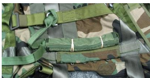
Figure 12.6bg – Securing the HPT Lowering Line
