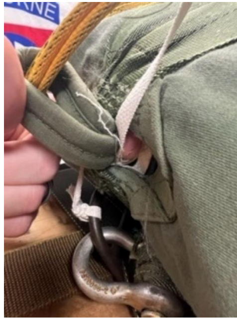
Figure 12.23c – Routing 1/4" cotton webbing
