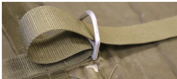
Figure 12.21a – Routing the Main Cargo Strap through the V-ring
