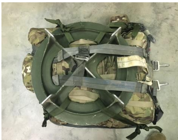
Figure 12.16u – HSPR laid out on the M7 Large Baseplate
