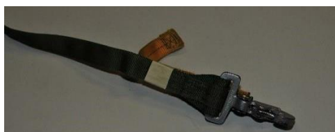
Figure 12.5b – Taping Yellow Safety Lanyard
