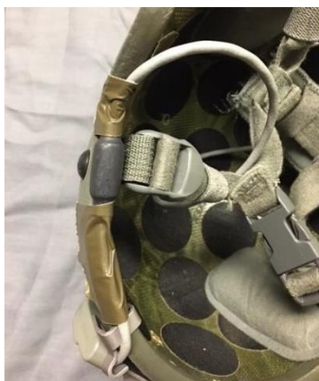
Figure 12.2f – Taping Wire and Coupling
