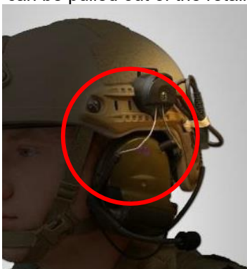
Figure 12.2j – Securing PTT Cable
