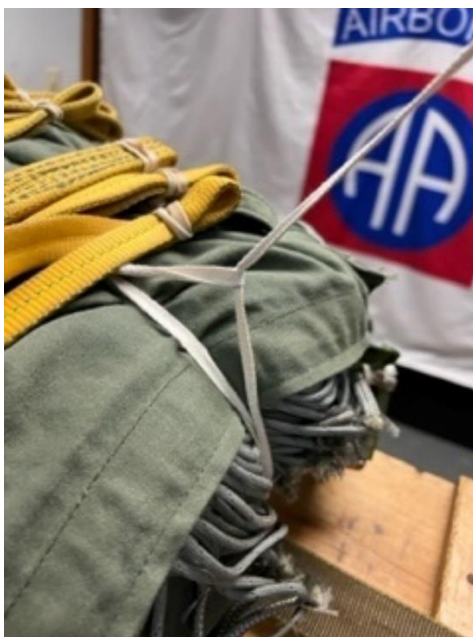
Figure 12.23l – Routing 1/4" cotton webbing through loop in the 1/4" cotton webbing
