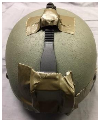
Figure 12.2g – Taping Wiring Harness
