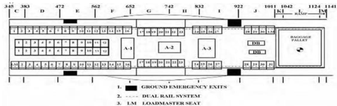
Figure 4.8e – Seating for In-flight Rigging, C-130J-30
