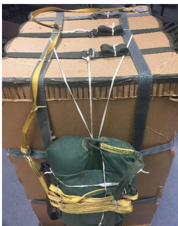
Figure 12.26f – Load Bearing Support
