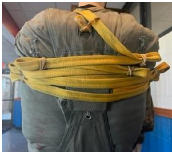
Figure 6.5b – Proper routing of USLM through stows and static line slack retainer bands
