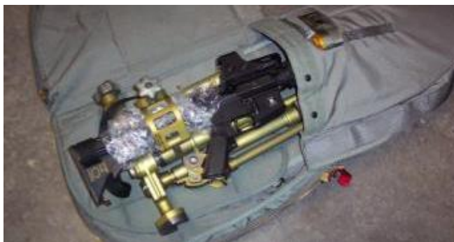
Figure 12.16r – M170A1 and M4 Rigged inside the MAWC
