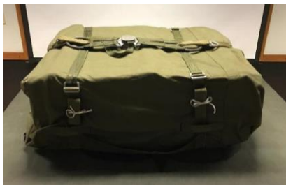
Figure 12.21c – A-21 Cargo Bag with Quick Release Assembly Attached
