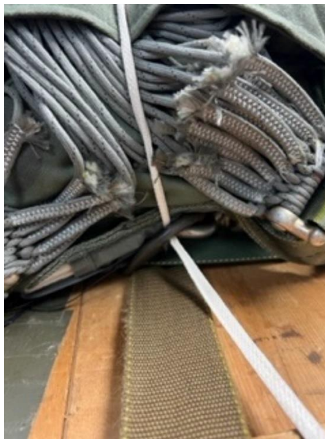
Figure 12.23k – Routing 1/4" cotton webbing around D-ring
