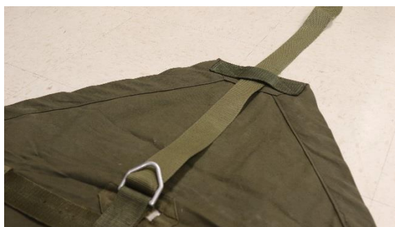
Figure 12.21b – Routing the Cargo Strap through the Strap Keeper
