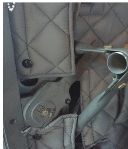
Figure 11.4f – Jump Platform Locking Pin in Groove
