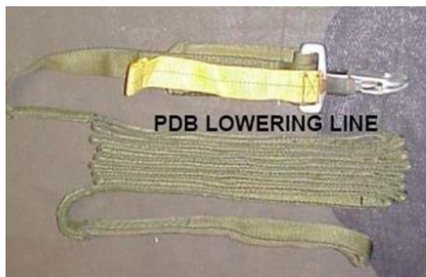
Figure 12.6av – PDB Lowering Line
