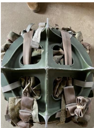
Figure 12.16t – Proper rigging of the M7 large baseplate with a MOLLE 4000
