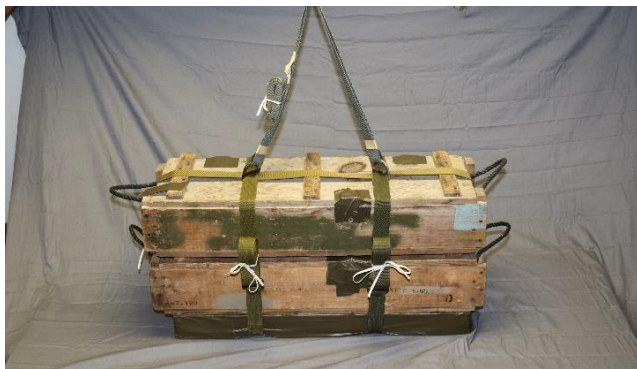
Figure 12.24a – A7-A Cargo Strap Prepared for the 68-Inch Pilot Parachute(s)
