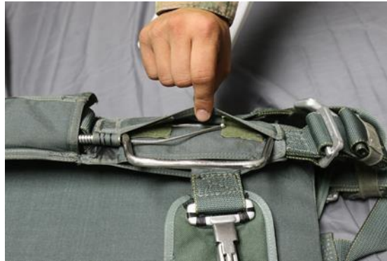
Figure 12.27d – Steel Swaged ball and Ripcord Housing Tacking
