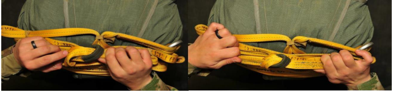
Figure G.4 – Inspection of the Girth Hitch of the 5 FT. USL
