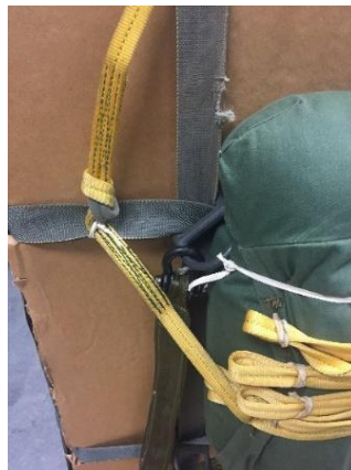
Figure 12.26j – USL Girth Hitch Tie-Down
