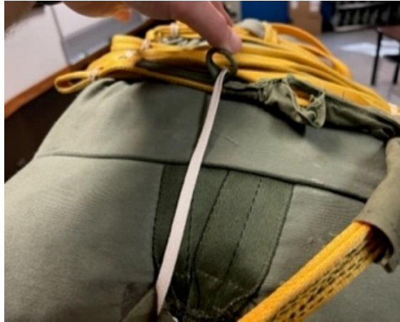
Figure 12.23f – Routing 1/4" cotton webbing through pack opening loop
