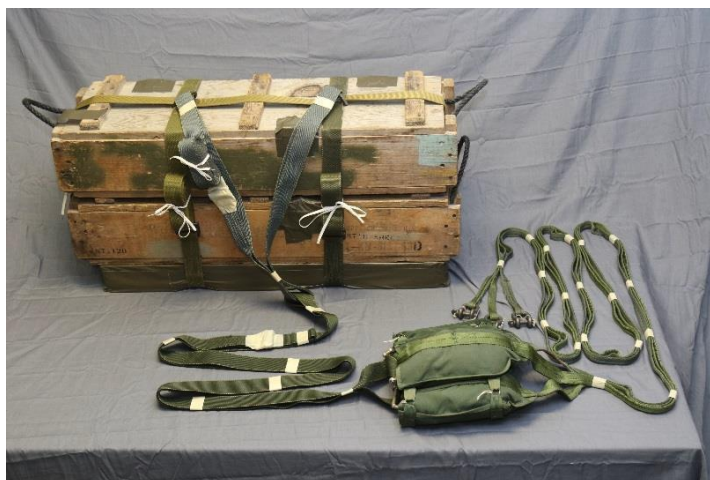
Figure 12.24b – Securing the 68-Inch Pilot Parachute(s) to the A7-A Cargo Strap
