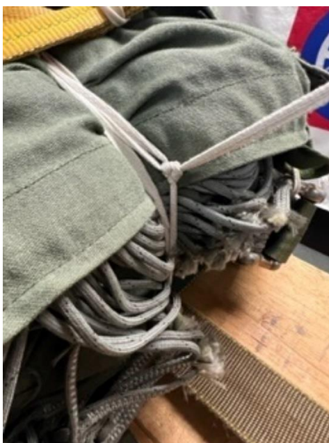
Figure 12.23m – Securing free running end of 1/4" cotton webbing with non-slip knot
