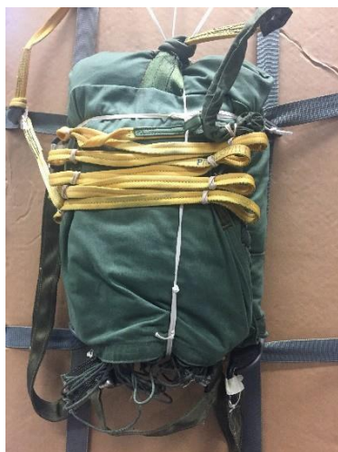
Figure 12.26g – 1/4" cotton webbing routing
