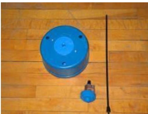
Combination mine M-21 Mine with tilt rod set up.
