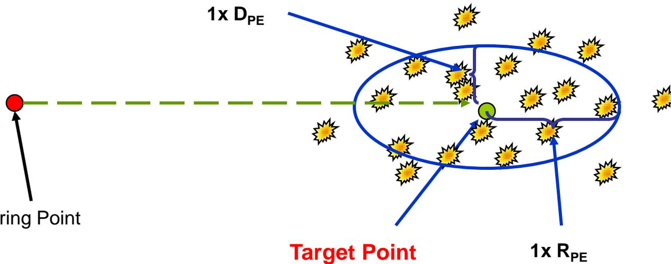
50% of rounds fired will land within one  $R_{PE}$  and one  $D_{PE}$  from the target point.
