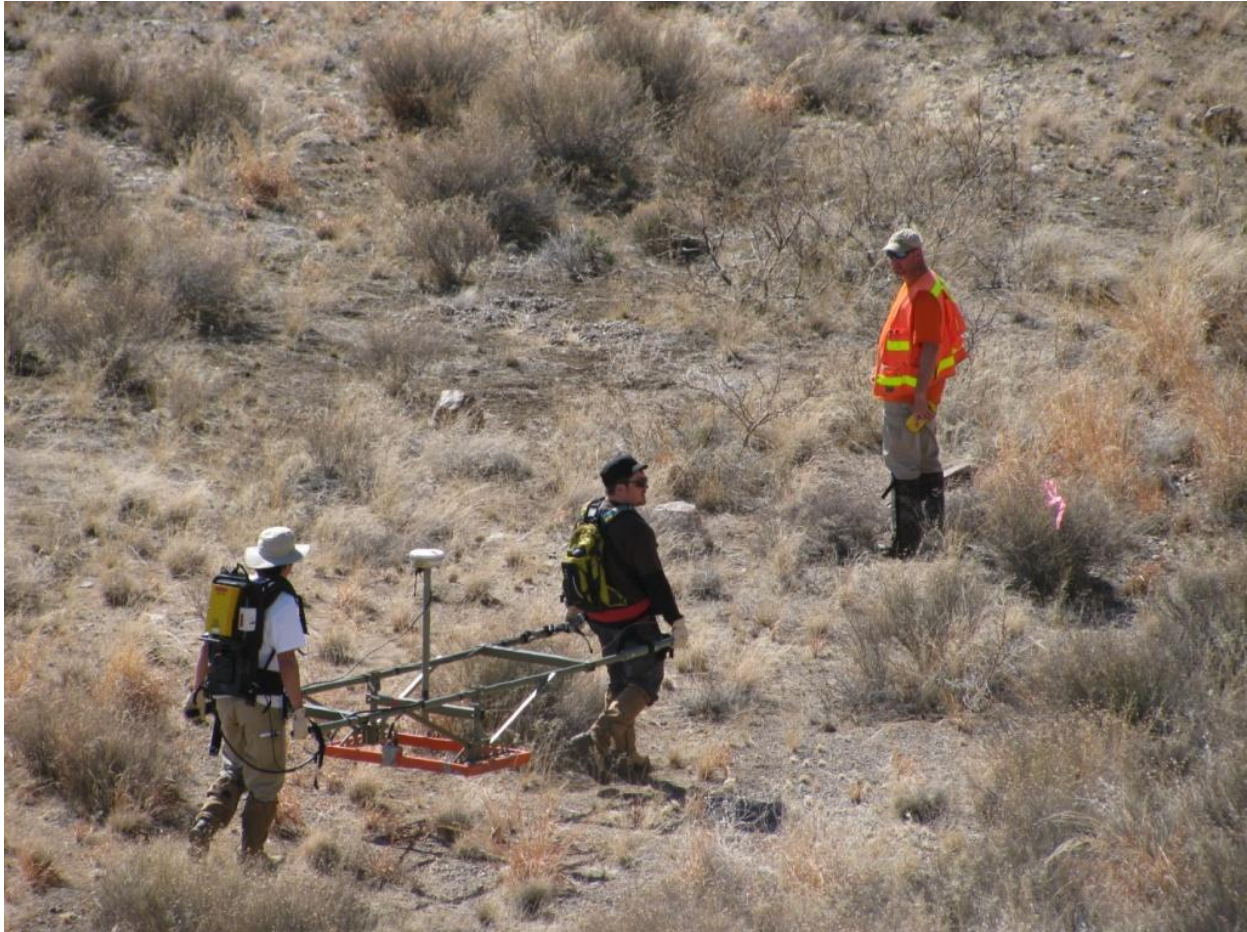
Figure 3-1. Man-portable DGM Data Collected Using EM61-MK2 in Litter Configuration
