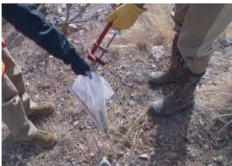
Fig1. Surface soil sampling on areas of suspected high MC concentration.
