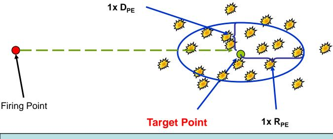
50% of rounds fired will land within one  $R_{PE}$  and one  $D_{PE}$  from the target point.
