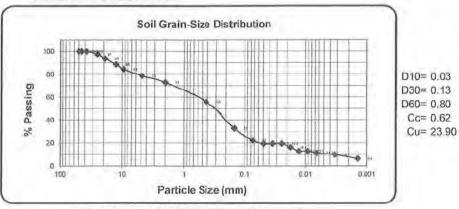
Test Method: ASTM D 2487 - Soil Class: SC
