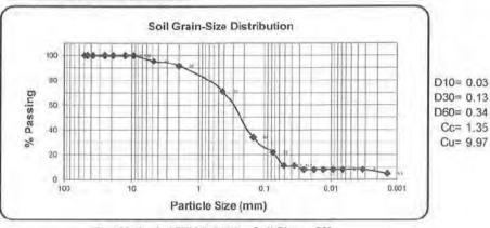
Test Method: ASTM D 2487 - Soil Class: SM
