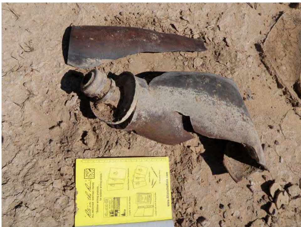
Photograph 5-2: Rotating band and fragments from 4.2-inch mortar shell(s) (October 7, 2010)
