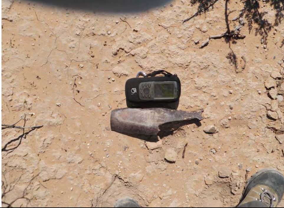
Photograph No. 103 Date: 10/7/2010 Time: 12:43 Site: Former Maneuver Area – Area 4 Description: Large fragment from 4.2-inch M2 mortar shell without rotating band
