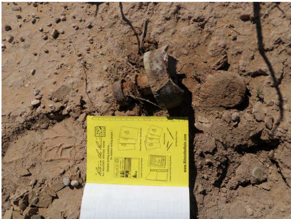
Photograph 5-1: Obturator/rotating band from 4.2-inch mortar shell (October 7, 2010)
