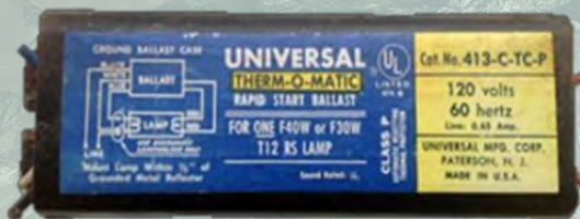
A typical pre-1979 PCB-containing fluorescent light ballast
