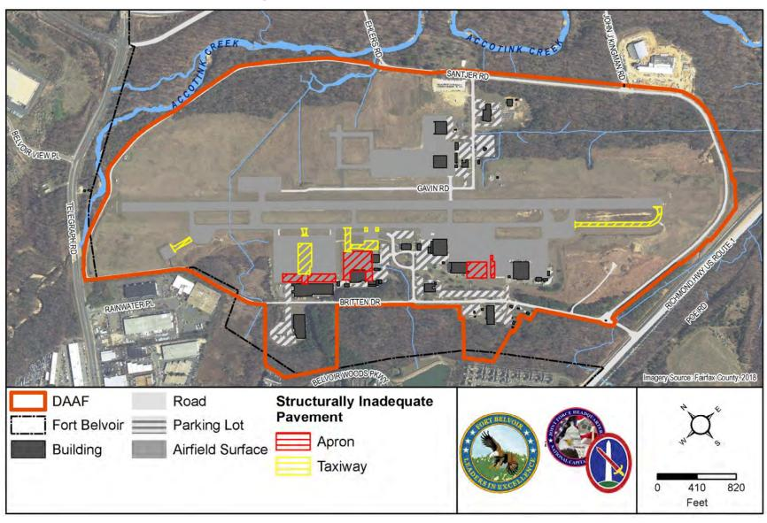
Figure 1.2-2: DAAF Airfield Pavement Conditions
