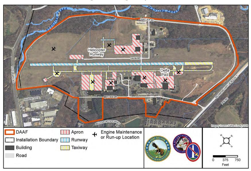
Figure 3.5-1: DAAF Engine Run-up Locations
