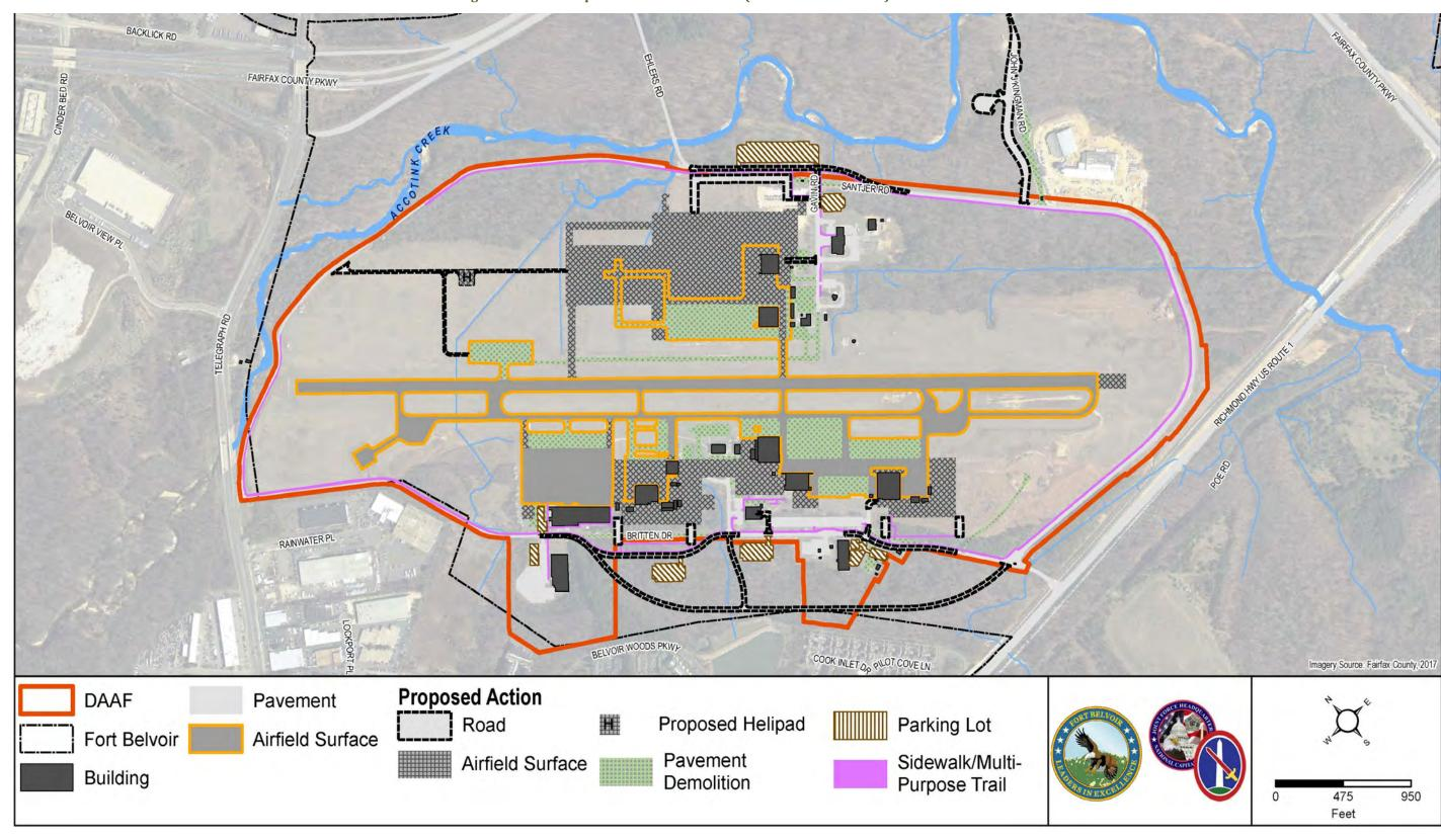
Figure 2.2-3: Full Implementation Alternative (Preferred Alternative) – New Pavement
