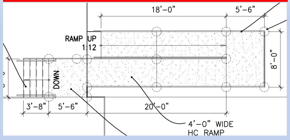
What is a side guard? A feature that does not allow a 4" sphere to penetrate. Prevents wheelchair casters from slipping off the edge of a 48" wide ramp.
