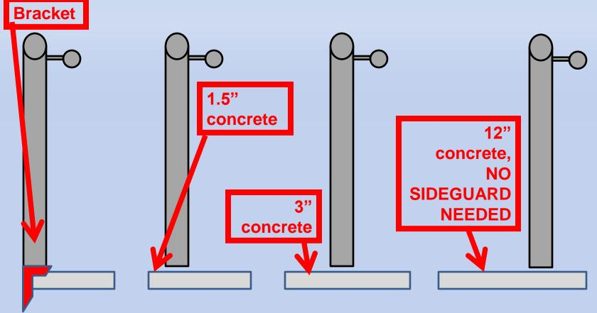
All ramps need 36" between handrails. Handrails and mounting bracket add another 6", for a minimum of 42 inches.
