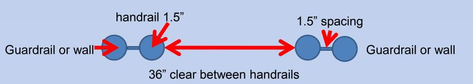
36+1.5+1.5+1.5= 42" absolute minimum width of ramp, assuming that the handrails are mounted to a wall
