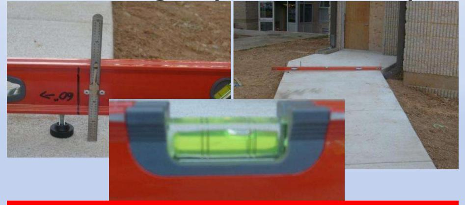
With the metal scale (ruler) set at 1 1/4" (60 inch ramp), the box level does not indicate a level condition. Resetting scale to 2 1/4 inches resulted in a level condition, exceeding permissable cross-slope.
