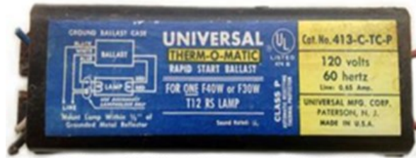
A typical pre-1979 PCB-containing fluorescent light ballast (FLB)
