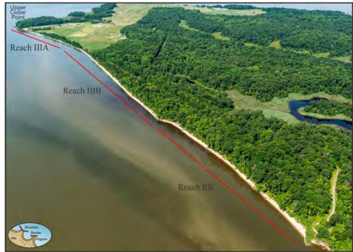
Figure 7-1. Reach III mainly consists of eroding forested upland banks except along Reach IIIA.
