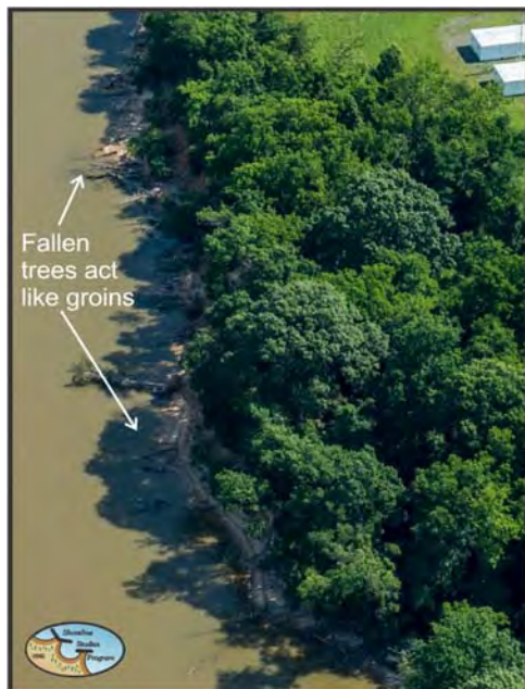
Figure 5-5. Photo showing how fallen trees can act like groins along the shoreline impacting alongshore sediment transport.
