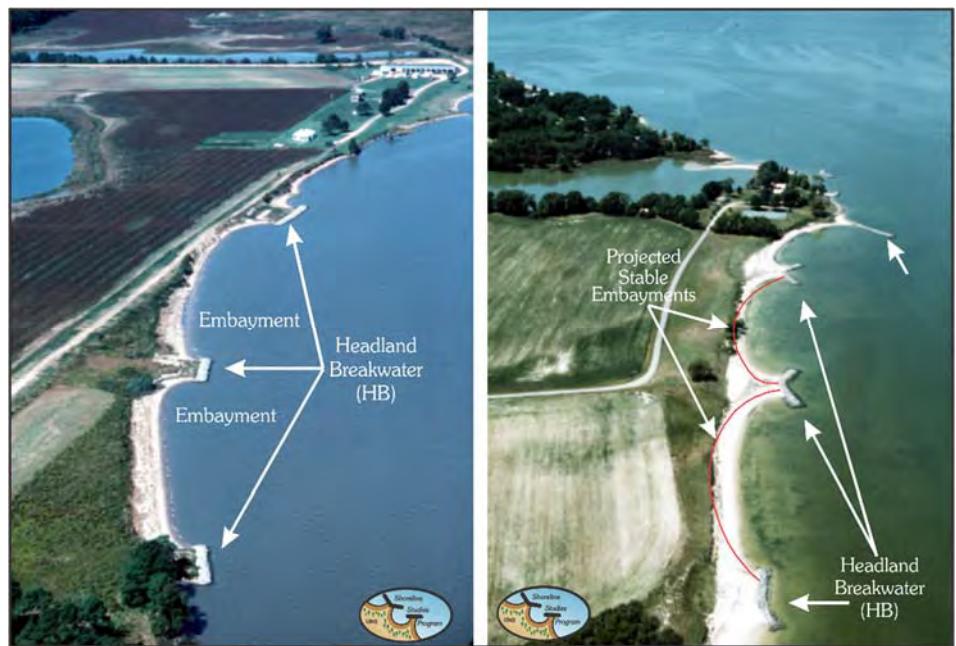
Figure 4-4. Examples of headland breakwaters spaced widely apart to allow adjacent shoreline to erode toward a dynamic equilibrium. This is a cost-effective shoreline management strategy when infrastructure is not threatened by the upland erosion between the structures. From Hardaway and Byrne (1999).
