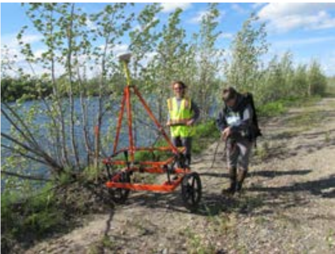
15) EM61 instrument equipped with survey-grade GPS rover collecting data along site access road.
