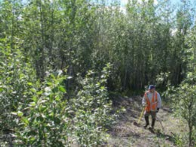
7) SUXOS using Schonstedt to clear study area prior to work.
