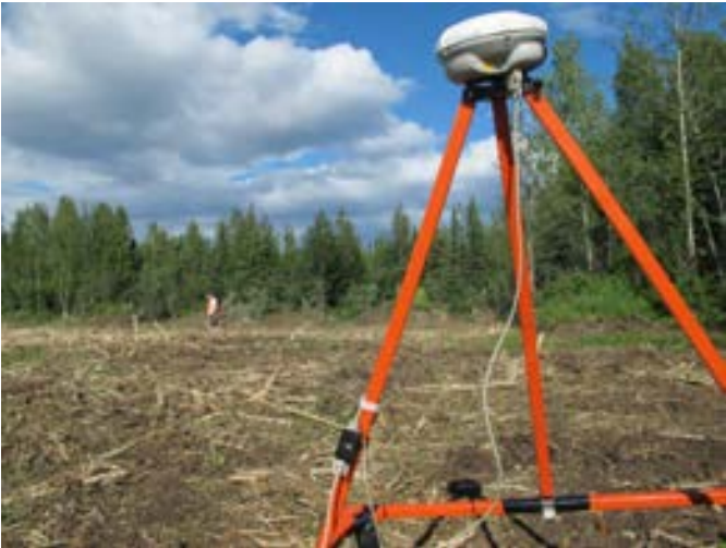
14) EM61 instrument equipped with survey-grade GPS rover.
