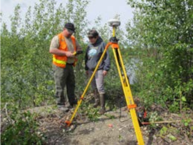
13) Survey base station set over control point on soil material stockpile shown in photograph 4.
