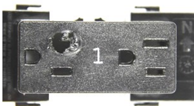
Receptacle damage from a loose connection.
